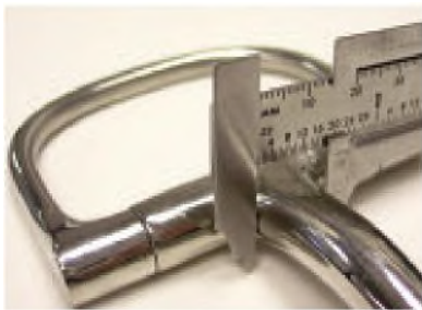
Diameter of bit is measured at the rings or cheeks of the mouthpiece.
