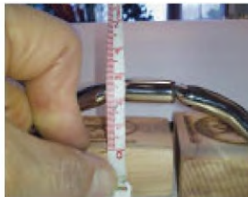
Measurement of a saffle bit to allow tongue relief. The maximum height of deviation is 30 mm from the lower part of tongue side to the highest part of deviation. The widest part of the deviation must be where the mouthpiece contacts the tongue and must have a minimum width of 30 mm.
